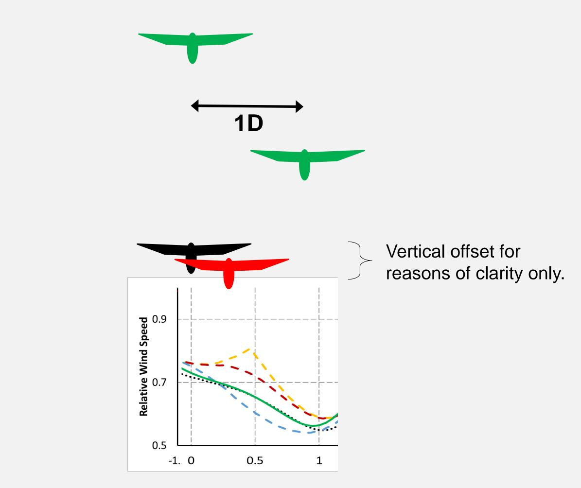
Figure 2: Illustrating how the choice of wake recombination impacts the "optimum" location of downstream wind turbines. The black turbine is the optimum location when using WakeBlaster. The red turbine is the optimum location when using analytical superposition of multiple wakes.
