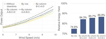
Figure 4: (left) Power produced in different maintenance schedules against a wind speed linearly increasing over time; (right) energy yield produced by various maintenance schedules compared to energy yield without downtime. Order of shutdown by column is indicated where "A-B-C-D" is in order from West to East.
