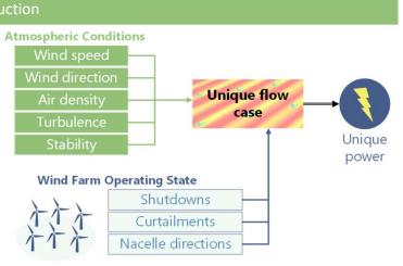
Figure 1: The factors that WakeBlaster considers in the simulation of 10-minute mean power
