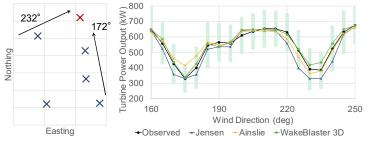
Figure 2: (left) The layout of wind turbines with the study turbine marked in red; (right) the power output of the study turbine in three different wake models compared to the observational medians (observational standard deviations are marked as grey bars).
